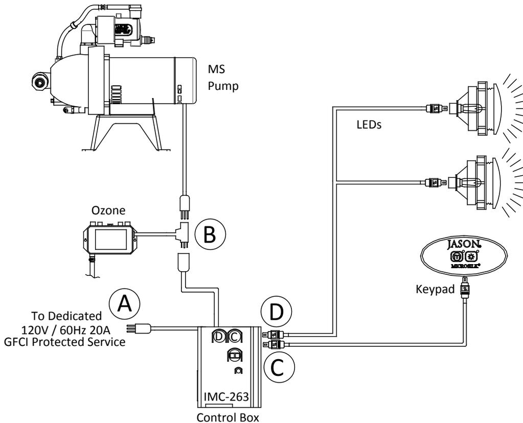
**NOTE:** This diagram also applies to 50 Hz, 240V pumps, controls, and power supply systems. Except that the MicroSilk® Pump junction boxes must be connected into one dedicated 240V, 20 amp GFCI circuit.
